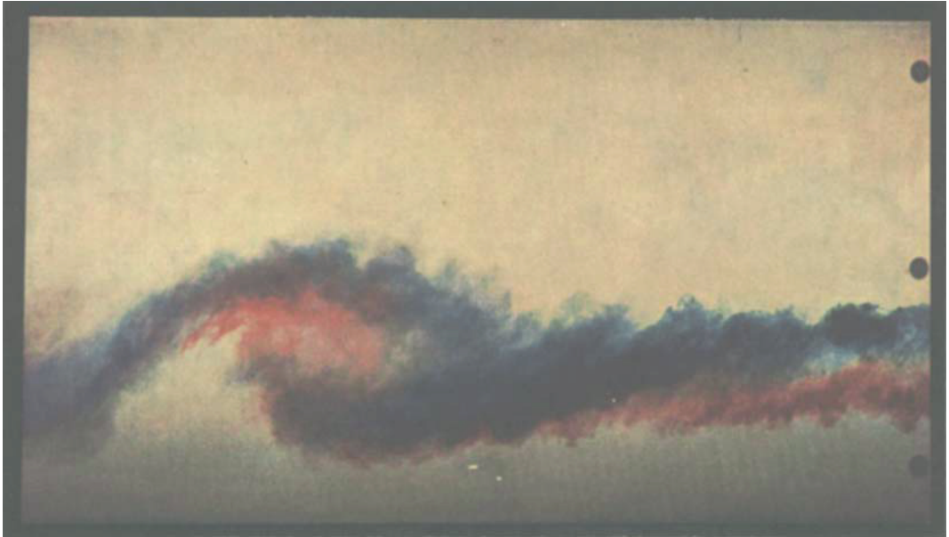
FIGURE 5. Flow as in figure 4. Simultaneous injection from both sides (blue dye from low-speed side, red dye from high-speed side).
